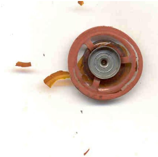
Figure 4 Diaphragm assembly, bottom (oil) side
