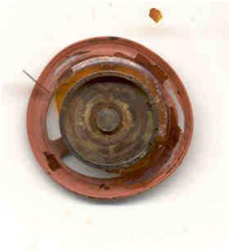
Figure 3 Diaphragm assembly – top (no oil) side
