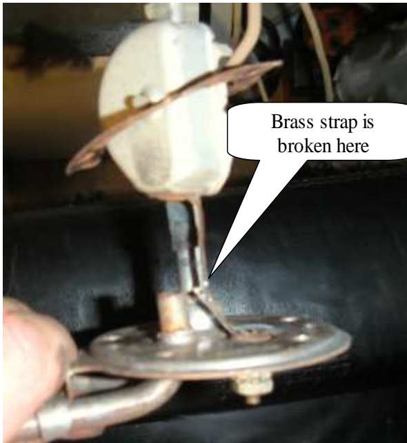
Photo 1 – broken strap on fuel sender
