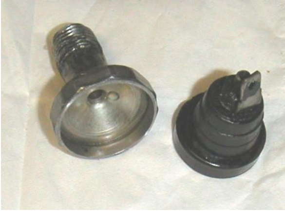
Figure 2 - The exterior parts of the switch
